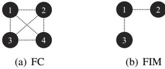
Fig. 2. Example topologies' conflicting graphs. Vertices are the links in interference graphs; dotted lines represent interference; (a) FC with 4 links; (b) FIM with 2 outer links.
