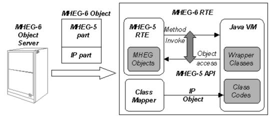
Fig. 3. Architecture of a MHEG-6 RTE
