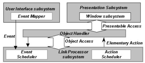
Fig. 4. Architecture of a MHEG-5 RTE
