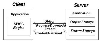
Fig. 2. Client/Server environment using MHEG
