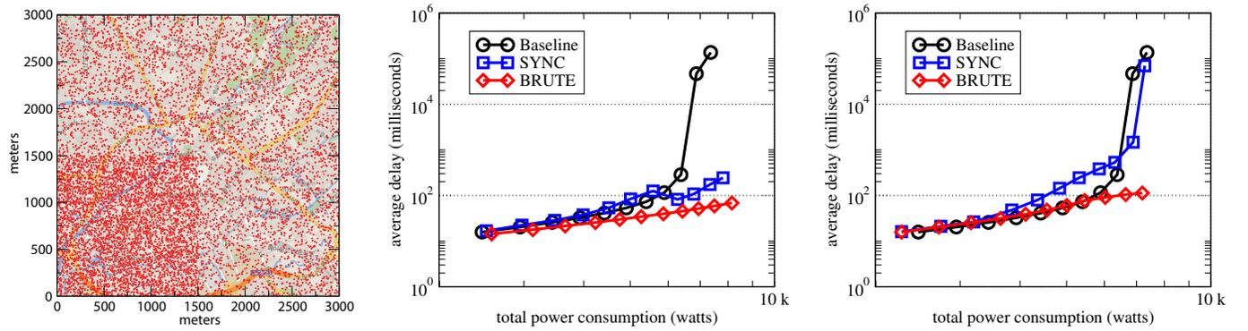
(a) Another heterogeneous user setup, where 5,000 users are distributed within  $1.5 \times 1.5$  km and rest 5,000 users are distributed elsewhere. (b) The delay-energy performance in the heterogeneous setup in Fig. 7(a), when the flow arrival is fixed and the average flow size varies from 100 to 300 kbits with 20 kbits step. (c) The delay-energy performance with the same setup as Fig. 7(b) except for  $\eta = 10$ .
