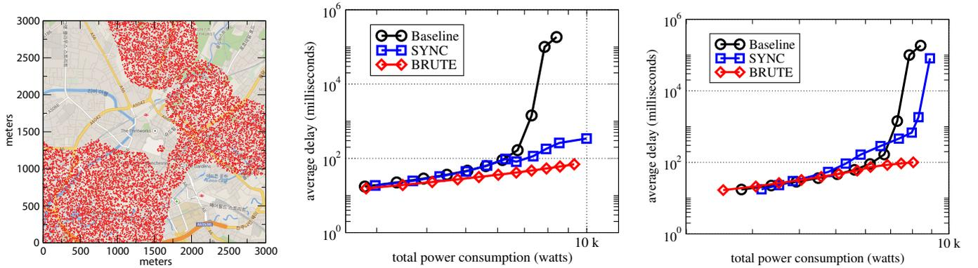
(a) An extremely heterogeneous user setup, where the users are placed only next to the BSs indexed with even numbers. (b) The delay-energy performance in the heterogeneous setup in Fig. 6(a), when the flow arrival is fixed and the average flow size varies from 100 to 300 kbits with 20 kbits step. (c) The delay-energy performance with the same setup as Fig. 6(b) except for  $\eta = 10$ .
