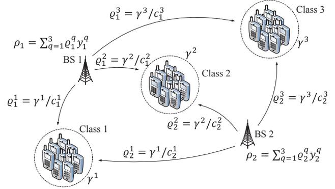
Fig. 1. System model and notations.
