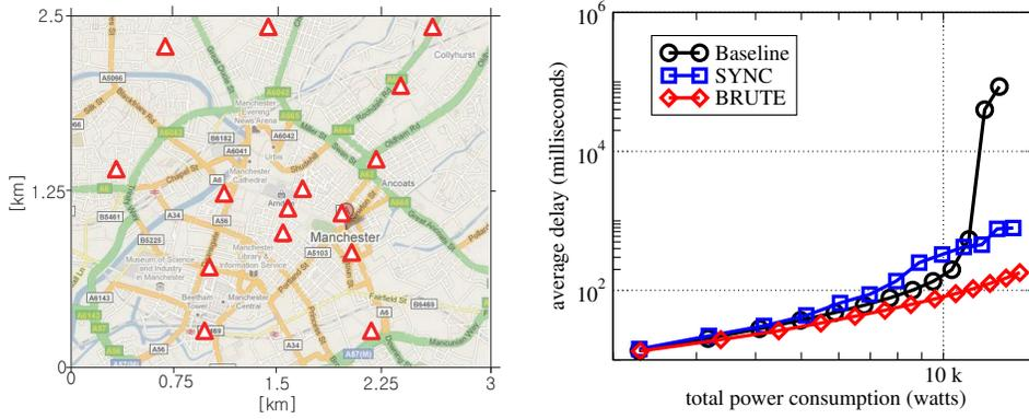
(a) A 3 km  $\times$  3 km real macro BS map (15 BSs) in Manchester, United Kingdom for our simulation. (b) The delay-energy performance in a homogeneous traffic scenario when the flow arrival rate is fixed and the average flow size varies from 100 to 580 kbits with 40 kbits step.
