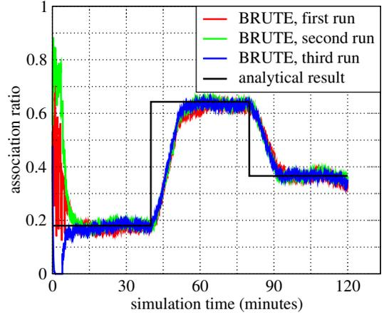
Fig. 4. The ratio of users on cell boundary which selects each BS. The ratio close to 1 indicates the more portion of boundary users are associated to BS 1. The solid black line indicates the analytically optimal association ratio. The flow arrival rate of the users close to BS 2 is changed to  $1.5 \times 10^{-2}$  and  $1.2 \times 10^{-2}$  flows/sec in 40 minute and 80 minute epoch, respectively.
