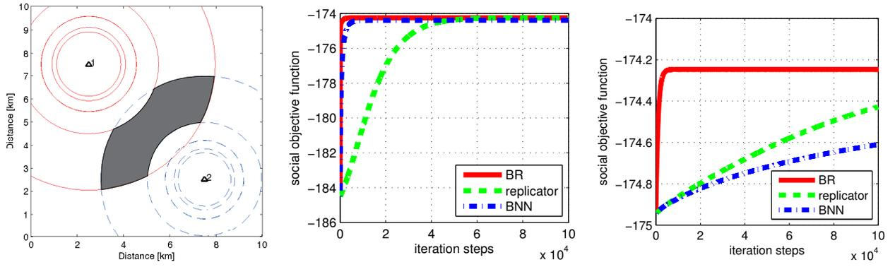
(a) Two cell scenario. The red solid and blue dashed lines represent the coverages of BSs 1 and 2, respectively. The shaded region represents the tie region between BSs 1 and 2. (b) Case I: The initial association ratio in the shaded tie region in Fig. 2(a) is 1%-99%. (c) Case II: The initial association ratio in each of the non-shaded regions in Fig. 2(a) is 50%-50%, and the initial association ratio in the shaded tie region is 20%-80%.
