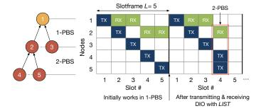
Fig. 4: An example of PAAS slot scheduling with a simple tree having height 2 and two child nodes for nodes 1 and 2. Initially all nodes are scheduled as 1-PBS. After transmitting and receiving the DIO includes LIST, the node 2 reschedules its RX slot and node 4 and 5 reschedule its TX slots as 2-PBS.
