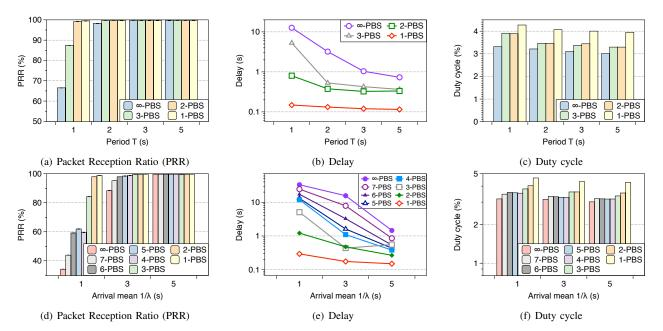
Fig. 5: Micro benchmark for Periodic and Poisson traffic with 1 receiver and 4 or 8 senders. It shows PRR, delay and duty cycle performances of n-PBS from 1-PBS to  $\infty$ -PBS.
