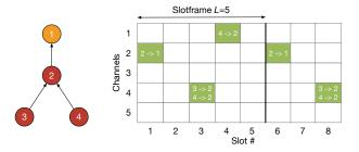
Fig. 2: Slot scheduling with channel hopping in TSCH.
