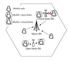
Fig. 1. Femtocell services: mobile-only, mobile+open femto, and mobile+closed femto
