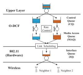
Fig. 1. Queue structure of O-DCF.
