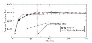
Fig. 10. Aggregate throughput traces and convergence times for W(x)=x and  $W(x)=\log\log(x+e)$
