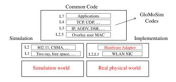
Fig. 2. Common Code Architecture: GloMoSim simulation codes are reusable in WiMesh without modification.
